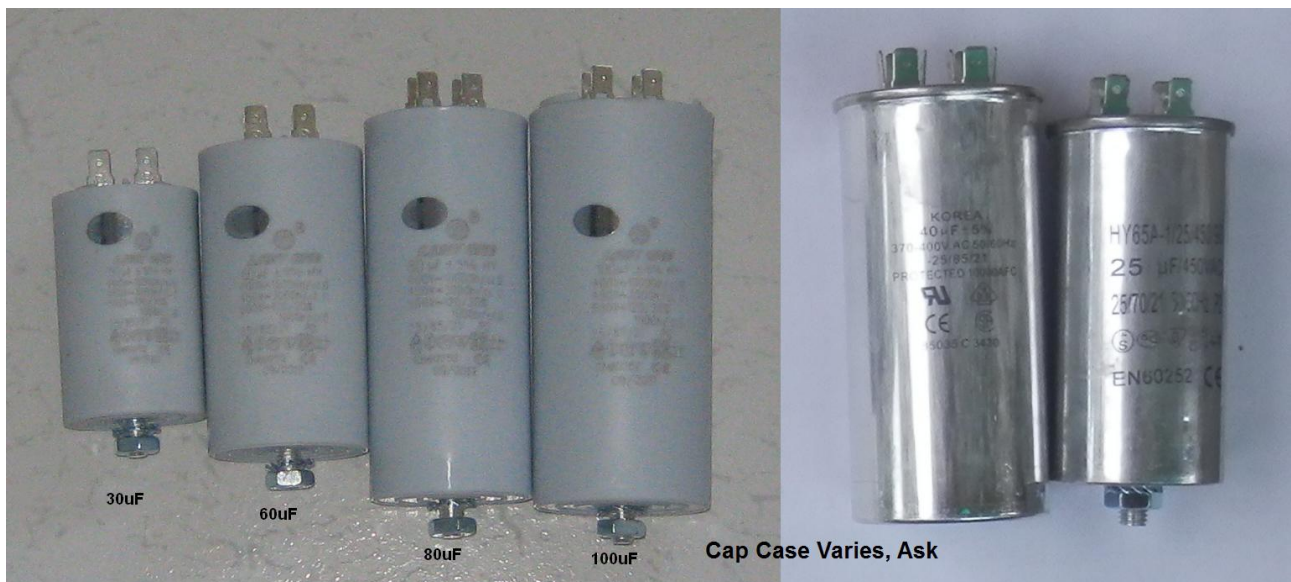
Illustration 3: Some Large Capacitors 25uF to 100uF
